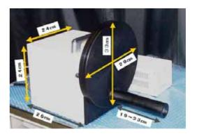
Figure 2 16band Multispectral camera
