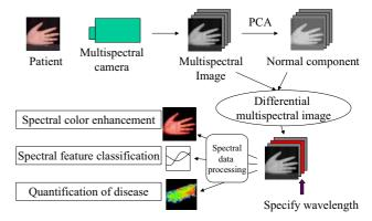
Figure 10 Proposed algorithm for multispectral skin color analysis.
