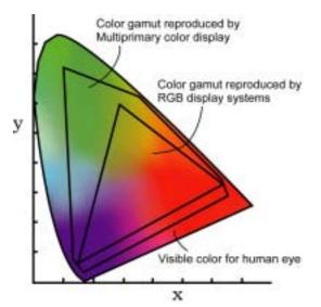
Fig.3 The concept of gamut expansion by multiprimary-color display
