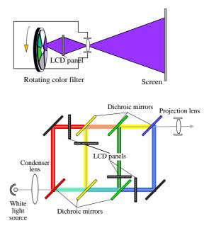
Fig.4 The examples of optical systems for multiprimary color projection display
