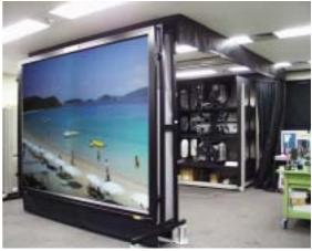
Fig.6 Six-primary 2x2 multi-projection display system with about 2300x2000 resolution
